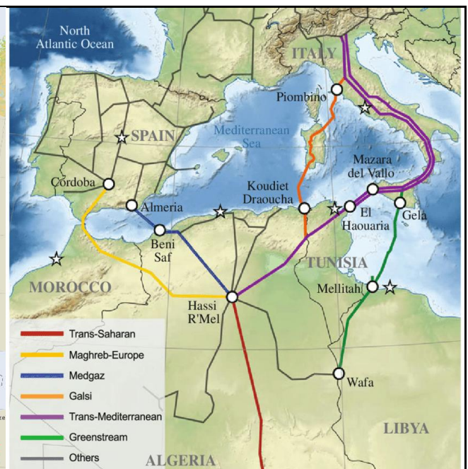
Scheme map 2. Submarine pipelines in the Mediterranean Sea, which supply gas from Algeria to Spain and Italy.
